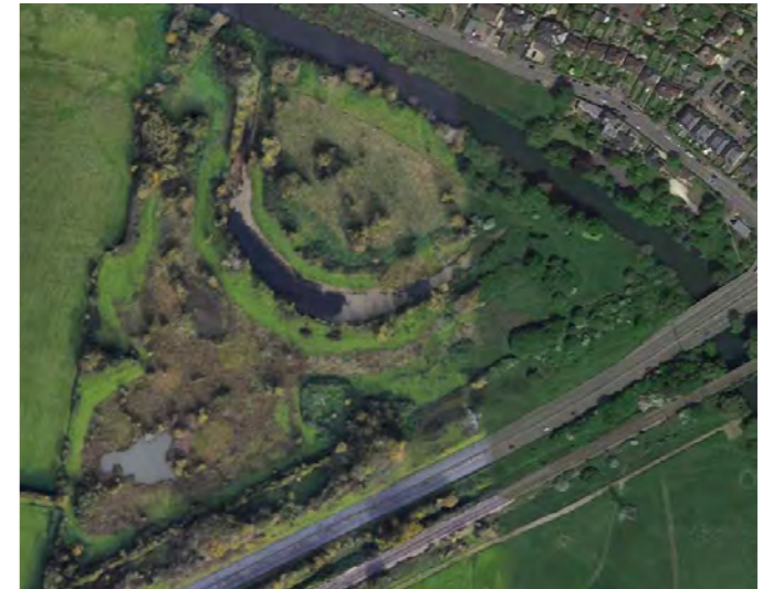
Attenuation pond and meander at Batheaston, River Avon. Ecological features include scrapes, wetland and scrub mosaic. The feature takes run off from the A4 Batheaston Bypass. ©2019 Google
